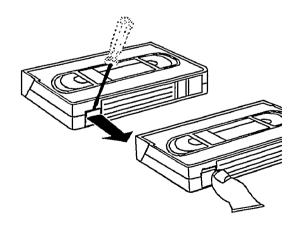
So that you don't accidentally delete an important recording, you can remove the special tab (erase protection) on the narrow side of the cassette with a screwdriver.
